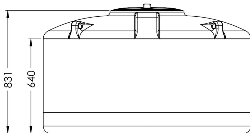
Tank capacity (Flange line) - 985L
